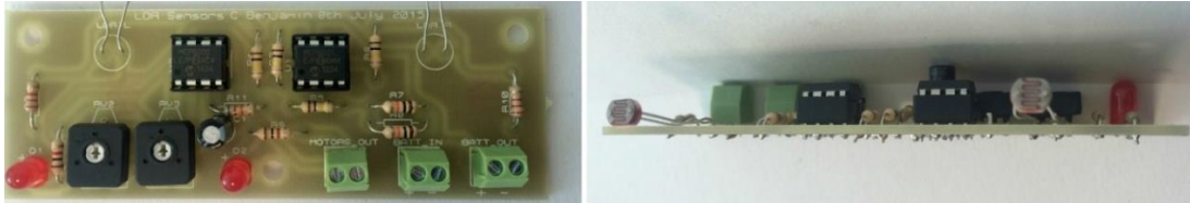
Fig 1. PCB 1 (LDR Sensor circuit) before feedback. Fig 2. Variety in solder thickness from side view.
